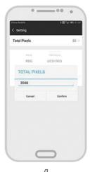
If pattern on Device is not even adjust Pixel # to total # of LEDs.
